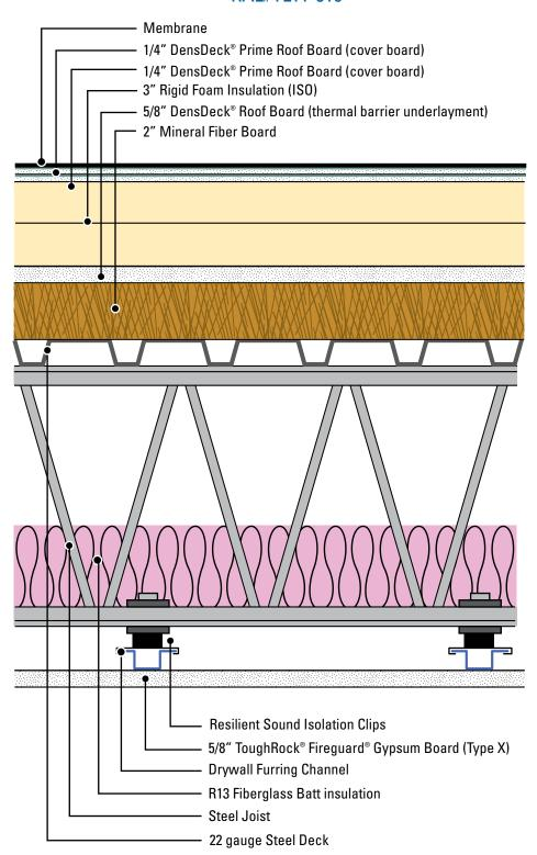
Tests per ASTM E 90 and ASTM E 413, were conducted in 2011 at Riverbank Acoustical Laboratories. Results are based on characteristics, properties and performance of materials and systems obtained under controlled test conditions. Actual results may vary.
