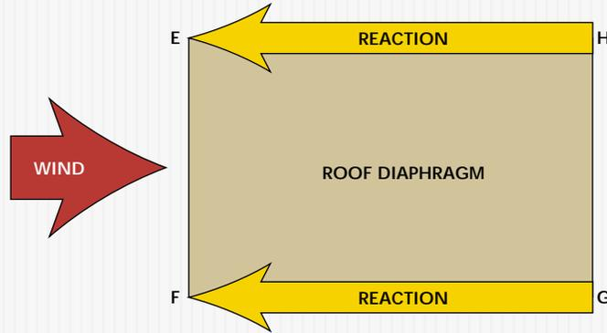
FIGURE 3a Roof to wall connections – fasteners must be able to transfer forces between roof and walls
