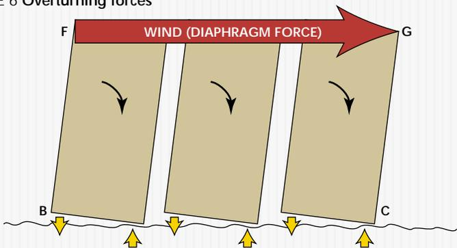
FIGURE 6a Holddown anchors - transfer overturning forces into foundation
