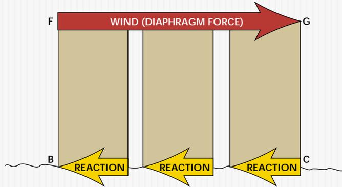
FIGURE 5a Shear wall anchor bolts - transfer shear forces into foundation
