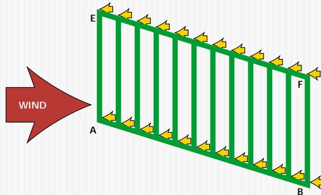
FIGURE 2a Perimeter anchor bolts – transfer forces into foundation
