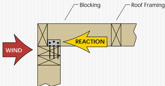
The transfer of forces into the foundation is accomplished by the perimeter anchor bolts which are loaded perpendicular to the grain of the bottom plate. The second half of the load transfers to the rafters and from these the force flows into the diaphragm (Figure 2b).
