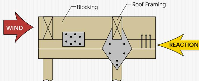
FIGURE 4 Shear wall reaction to lateral loads
