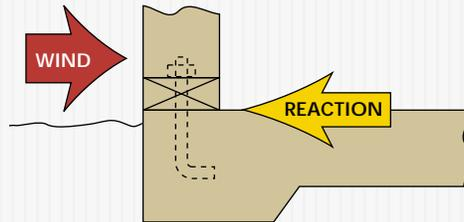
FIGURE 2b Rafter connection detail – transfers forces into diaphragm
