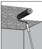
**Tools:** Stipple Paint Roller, Hand Extension, Roller Pan
