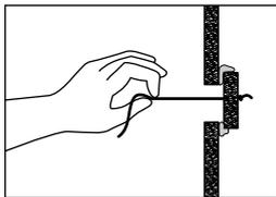
1. Cut out a rectangle around damaged area with knife or keyhole saw.
