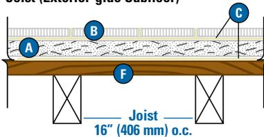
**DensShield Tile Backer Over Engineered Joist (Tongue-and-Groove Subfloor)**
