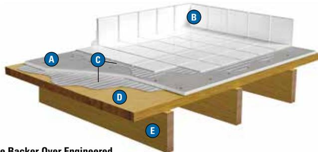
**DensShield Tile Backer Over Conventional Joist (Exterior-glued Subfloor)**
