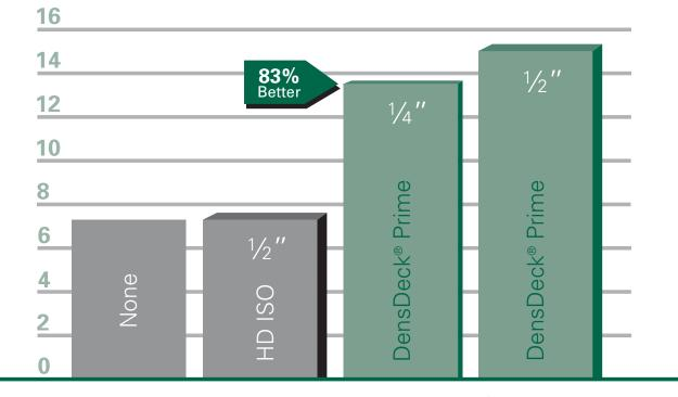
Thermoplastic membranes tested in assemblies with ¼" DensDeck<sup>®</sup> Prime boards underneath were **83 percent more puncture-resistant** than membranes with ½" HD ISO or with no cover board at all.<sup>[1]</sup>\*
