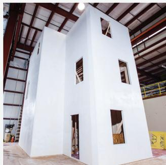
Trial 2: Fluid-Applied Membrane WRB-AB System
